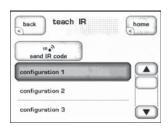
The Teach IR page displays a scrolling list of all the available IR codes in the SSP-800 Surround Sound Processor. Simply scroll to the command you want your macro-capable remote to learn and touch the **Send IR Code** button. The SSP-800 continuously sends the appropriate command code via the front panel - as long as the button is pressed – until your third-party remote control has learned it.
